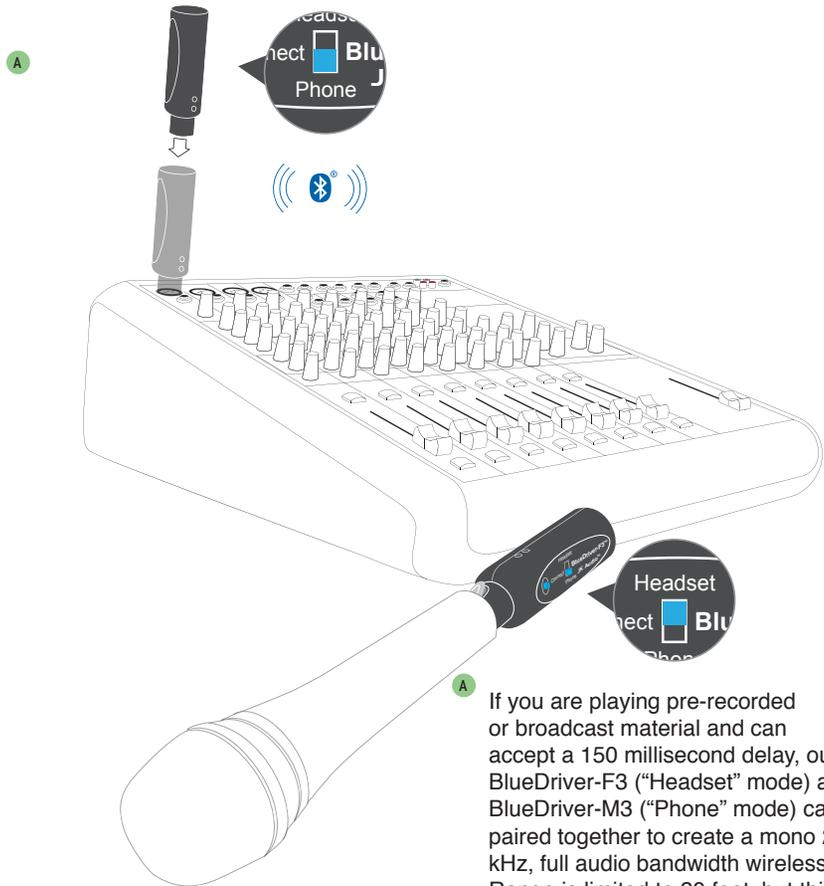
**A** If you are playing pre-recorded or broadcast material and can accept a 150 millisecond delay, our BlueDriver-F3 (“Headset” mode) and BlueDriver-M3 (“Phone” mode) can be paired together to create a mono 20 kHz, full audio bandwidth wireless link. Range is limited to 30 feet, but this may be just enough for your application. A2DP is a one-way transmission, with nothing coming back on the return channel.
