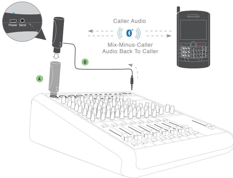
**A** Simply plug BlueDriver-M3 into any mic level input of your mixer or console. Pair to your cell phone and get ready to take calls as you normally would. This setup allows voice band bi-directional audio from your cell phone.
