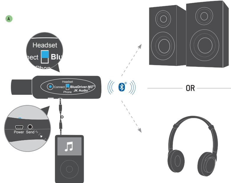
**A** Forget the XLR jack and jump right to the 3.5 mm socket. The "Headset" mode of BlueDriver-M3 connects to Bluetooth headphones or wireless speakers, and transmits full 20 kHz audio bandwidth Stereo A2DP audio. Simply connect the supplied cord between the SEND mini jack on your BlueDriver-M3 and the line level or headphone output jack of your audio
